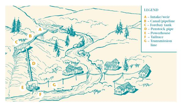
Picture of the plant structure taken from *Micro-hydropower Systems - A Buyer's Guide, Natural Resources Canada, 2004*
